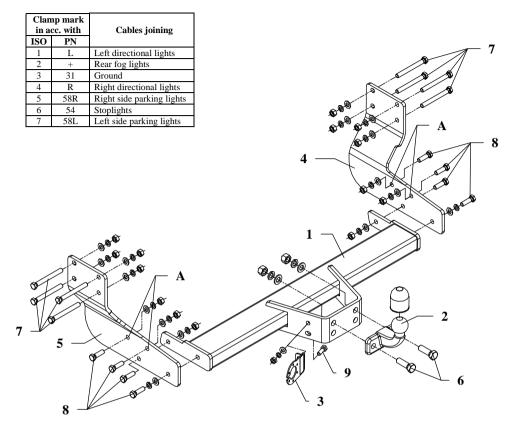
This towbar is designed to assembly in following cars: MERCEDES SPRINTER and VOLKSWAGEN CRAFTER, 3,25/3,665/4,325m, metal built-up, with step board, single wheels, produced since 04.2006, catalogue no. D34 and is prepared to tow trailers max total weight 3500 kg and max vertical load 150 kg.
