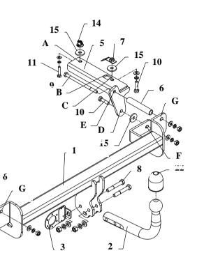
This towbar is designed to assembly in following cars: **OPEL ZAFIRA II**, produced since 2005, catalogue number **E48** and is prepared to tow trailers max total weight **1650 kg** and max vertical mass **75 kg**.
