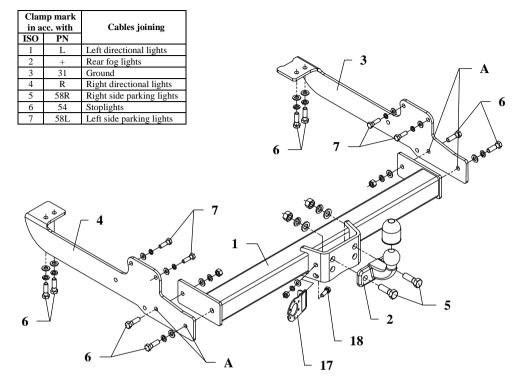
This towbar is designed to assembly in following cars: **RENAULT MASTER** and **OPEL MOVANO** (both loading platform) produced since 1998 till 03.2010, catalogue number **G36** and is prepared to tow trailers max total weight **2300 kg** and max vertical load **100 kg**.
