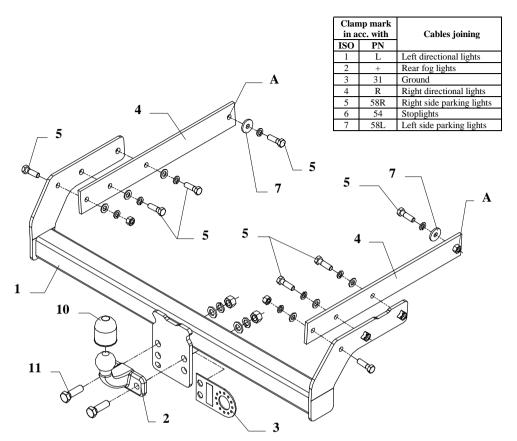
This towing hitch is designed to assembly in following cars: **VOLKSWAGEN T5–TRANSPORTER**, loading platform, produced since 01.2003, catalogue no. K47 and is prepared to tow trailers max total weight 2500 kg and max vertical load 100 kg.
