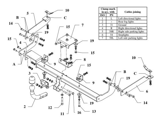
This towbar is designed to assembly in following cars: **CITROEN XSARA**, 3/5 doors, produced since 1997 till 2004, catalogue no. **P10** and is prepared to tow trailers max total weight **1300 kg** and max vertical load **70 kg**.
