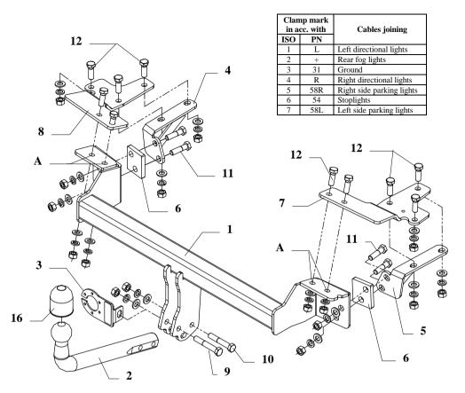
This towbar is designed to assembly in following car: **SUZUKI LIANA, 4 doors,** produced since 2002 till 2007, catalogue number **W20** and is prepared to tow trailers max total weight **1200 kg** and max vertical load **75 kg**.
