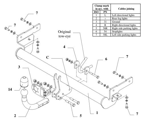
This towbar is designed to assembly in following car: MITSUBISHI CARISMA 4/5 door, produced since 08.1995 till 1999 and since 2000 till 2005, catalogue number Z23 and is prepared to tow trailers max total weight 1450 kg and max vertical load 75 kg.
